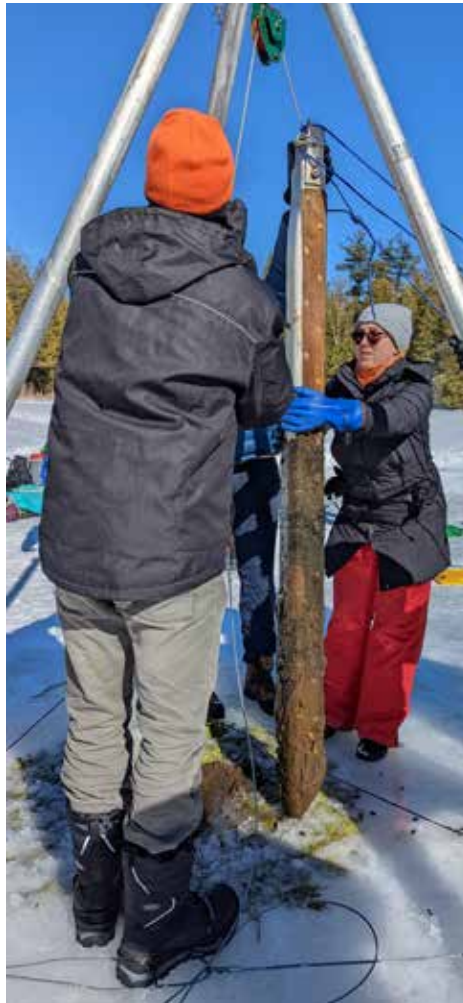
◀ The core sample of lake sediment being winched up out of the hole in the ice.
